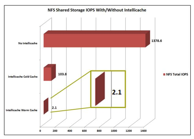
This chart shows how enabling IntelliCache reduces peak IOPS on shared NFS storage from 1378 to, at first, 103 IOPS, and then ultimately 2.1 IOPS.
