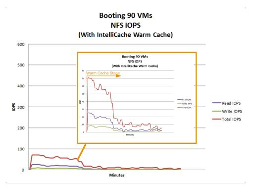
how, in the top graph, the initial spike in IOPS as the 90 VMs boot for the first time. As the Read Cache fills, the IOPS decrease significantly and continue to decrease as more data is cached. In the bottom chart, the 90 VMs were booted for the second time and there were significantly fewer IOPS because the cache was populated from the first boot cycle.\*
