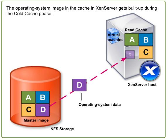
This illustration shows how, when a desktop VM cannot find part of its operating system in the Read Cache on the local host, the desktop VM accesses the master image on the storage. As the master image is read, the Read Cache is populated with part of the missing image. In this illustration, "D" represents a block of data not found in the Read Cache.
