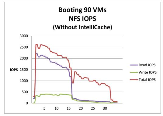
This graph shows the Read, Write and Total IOPS on the NFS storage as the NetApp Operations Manager recorded during the initial boot test we performed without IntelliCache enabled.<sup>4</sup>
