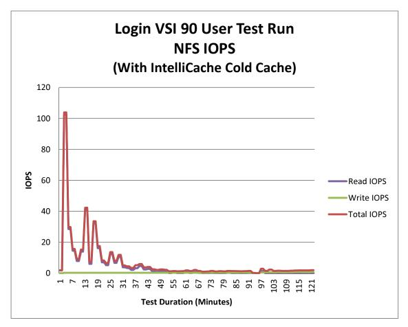
This graph shows that as the Read Cache fills up, after the first user connects to a desktop, the need to access data from shared storage falls (the load drops below 40 IOPS) and then continues to diminish. All writes are flat because with Pooled Desktops the desktop VMs write their data locally in the Write Cache and not on shared storage.
