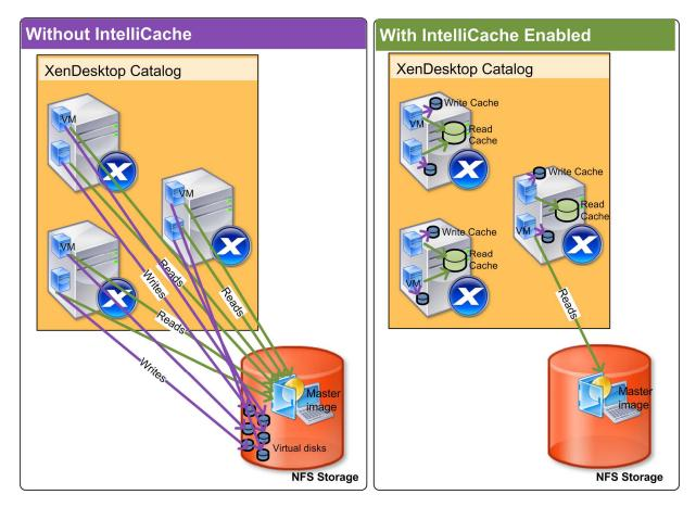
Without IntelliCache, each desktop VM reads data from the master image on the shared storage and writes data to its virtual disk on the shared storage. However, with IntelliCache enabled for Pooled Desktops, desktop VMs cache most read data locally, so they only need to read from the shared storage when data is not available in their local cache. Likewise, desktop VMs write to their own Write Cache on local storage.
