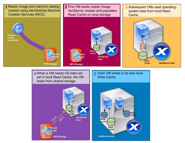
This illustration shows how IOPS are reduced, for Pooled Desktops, when VMs in the same machine catalog use IntelliCache. As shown in the last panel, all of the VMs read from the Read Cache.
